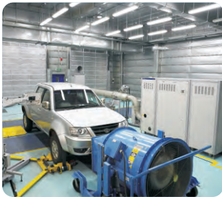
Chassis Dynamometer Test Cell
